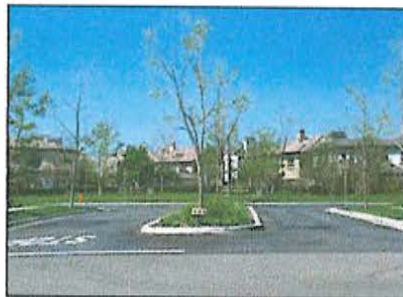
3.2.1.6 b) Raised planted medians calm traffic and provide a neighborhood entry feature.
